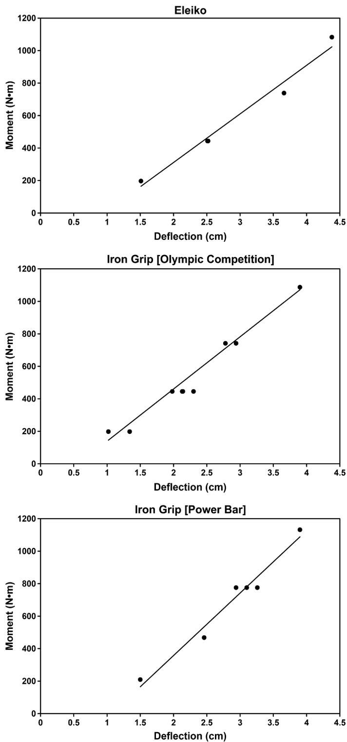
**Figure 3.** Plots to determine apparent stiffness for Eleiko, Iron Grip [Olympic Competition] and Iron Grip [Power] bars. Data are combined from the loading-unloading cycles. Because of the uniformity of data, some points may overlap.
