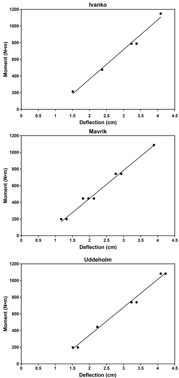
**Figure 4.** Plots to determine apparent stiffness for Ivanko, Mavrik and Uddeholm bars. Data are combined from the loading–unloading cycles. Because of the uniformity of data, some points may overlap.
