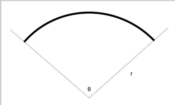
**Figure 6.** Alternative method to determine beam deformation.  $r$  = radius of arc formed by beam;  $\theta$  = angle formed by the 2 radii perpendicular to the ends of the beam.
