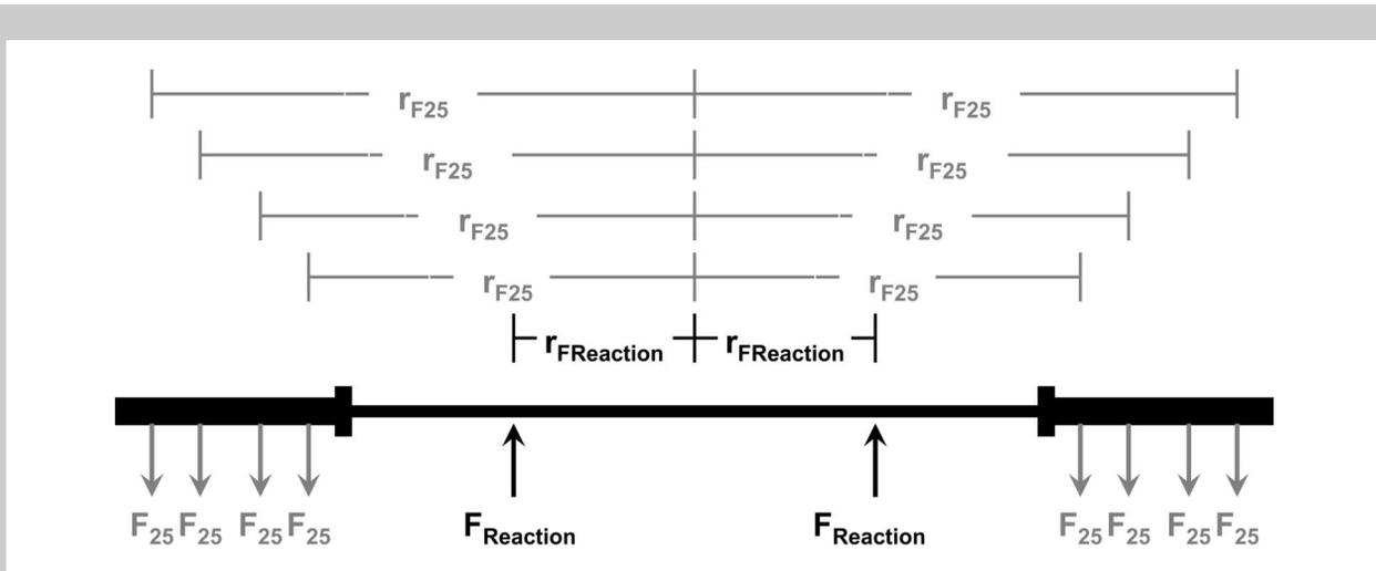
**Figure 2.** Free-body diagram to determine bending moments acting on the center of a bar.  $F$  = force;  $r$  = moment arm for force.
