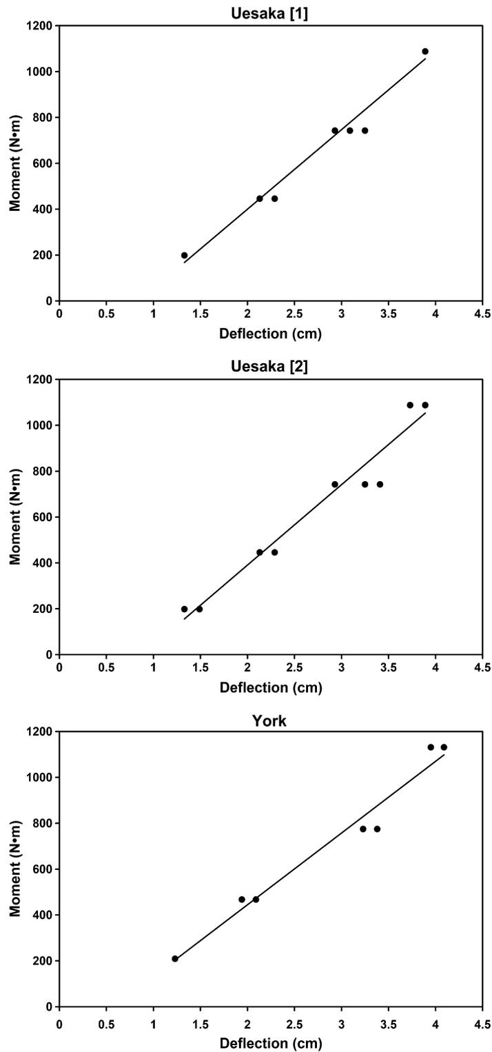
**Figure 5.** Plots to determine apparent stiffness for Uesaka and York bars. Data are combined from the loading–unloading cycles. Because of the uniformity of data, some points may overlap.
